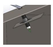
ATTACH THE SMALLER ROUND NUT AND ONE 50mm WASHER ONLY.PUSH THROUGH THE HOLE ON THE LIGHT PLATE ADJUST THE NUT AND WASHER PLACEMENT FOR BEST FIT.
