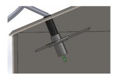
ATTACH ANOTHER 50mm WASHER. ON THE OTHER SIDE OF THE LIGHT PLATE AND USE THE LONGER NUT TO HOLD IN PLACE, THE END OF THE NUT SHOULD BE FLUSH WITH THE END OF THE LIGHT FITTING.
