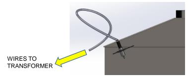
CONNECT 2x WHITE WIRES ON THE WIRING TO THE TRANSFORMER AND THE LIGHT WILL BE READY FOR USE
