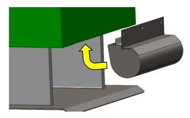
1. POSITION FAN ASSEMBLY ADJACENT TO THE REAR PANEL OF THE APPLIANCE, POSITION THE FAN IN BETWEEN THE CUT OUTS ON THE REAR PANEL. PUSH THE FAN ASSEMBLY AS HIGH AS ALLOWABLE.
