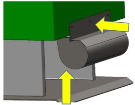
2. MAKE SURE THE HOLES ON THE FAN ASSEMBLY LINES UP WITH THE HOLES ON THE REAR PANEL
