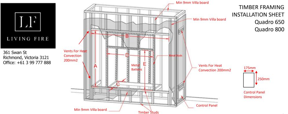
Unit stands on small legs that sit on framing/floor which provide sufficient clearance . Flexible connections descend from the middle of the unit to control panel.
