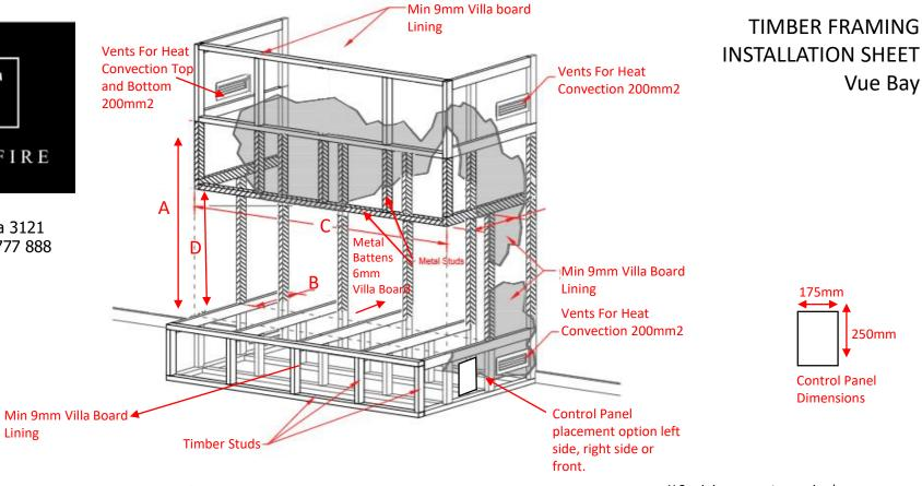
Unit stands on small legs that sit on framing/floor which provide sufficient clearance. Flexible connections descend from the middle of the unit to control panel.
