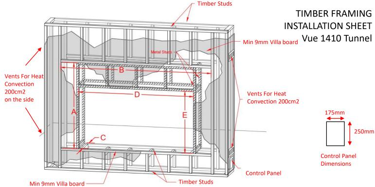
Unit stands on small legs that sit on framing/floor which provide sufficient clearance . Flexible connections descend from the middle of the unit to control panel. Fluing off unit located on the top left side of the unit please see spec drawing
