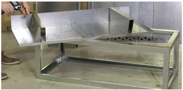
locate and secure the side panels to the base panels with self tapping screws ensuring the side panels are inside the base panel folds.
