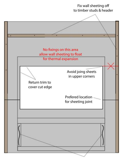
Self tappers & Selleys 401 RTV or similar can be used to secure wall cladding to the lower unit casing / framework
