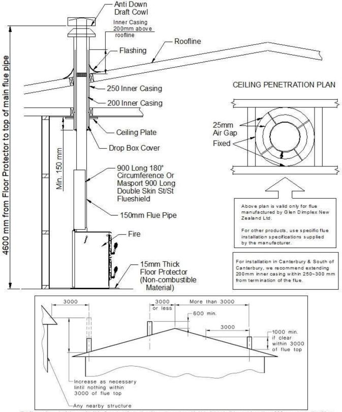
If a flue exits out of the roof within 3 meters from the ridge, the outer shield height shall be not less than 600mm above the ridge. If the flue exits further than 3 meters out from the roof ridge then it must project at least 1000mm above roof penetration. This dimension may need increased to ensure that the top of the flue is at least 3 meters away from the roof or other obstructions when measured horizontally.
