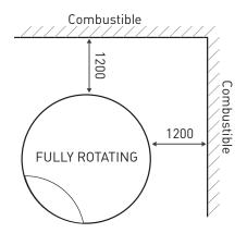
950mm minimum clearance is required if the rotation of the BathyscaFocus is locked at 120° or 90° away from the wall. Locking the BathyscaFocus so that the opening is fixed is an option available on purchase.
