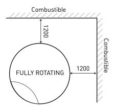
520mm minimum clearance is required if the rotation of the DomoFocus is locked at 120° or 90° away from the wall. Locking the DomoFocus so that the opening is fixed is an option available on purchase.
