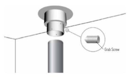
2. Engage the firebox with the bolt bearings as per the diagram below.
