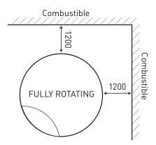
700mm minimum clearance is required if the rotation of the ErgoFocus is locked at 120° or 90° away from the wall. Locking the ErgoFocus so that the opening is fixed is an option available on purchase.
