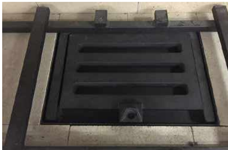
Figure 3) Ash Grate pictured in the fully-closed position.
