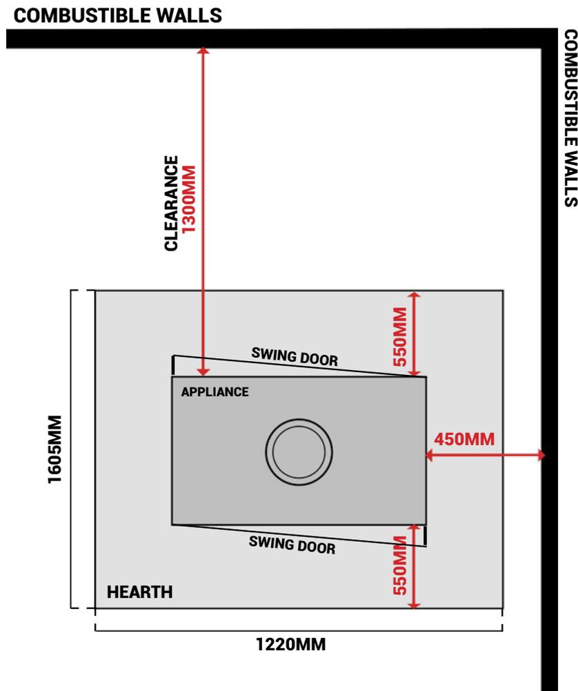
\*\*\*The appliance must be elevated a minimum of 250mm above the hearth(on a non combustable surface). If the heater is placed directly onto the hearth, the hearth dimensions required will be greater. Please refer to AS/NZS 2918:2001 as per the minimum for a non-tested appliance.
