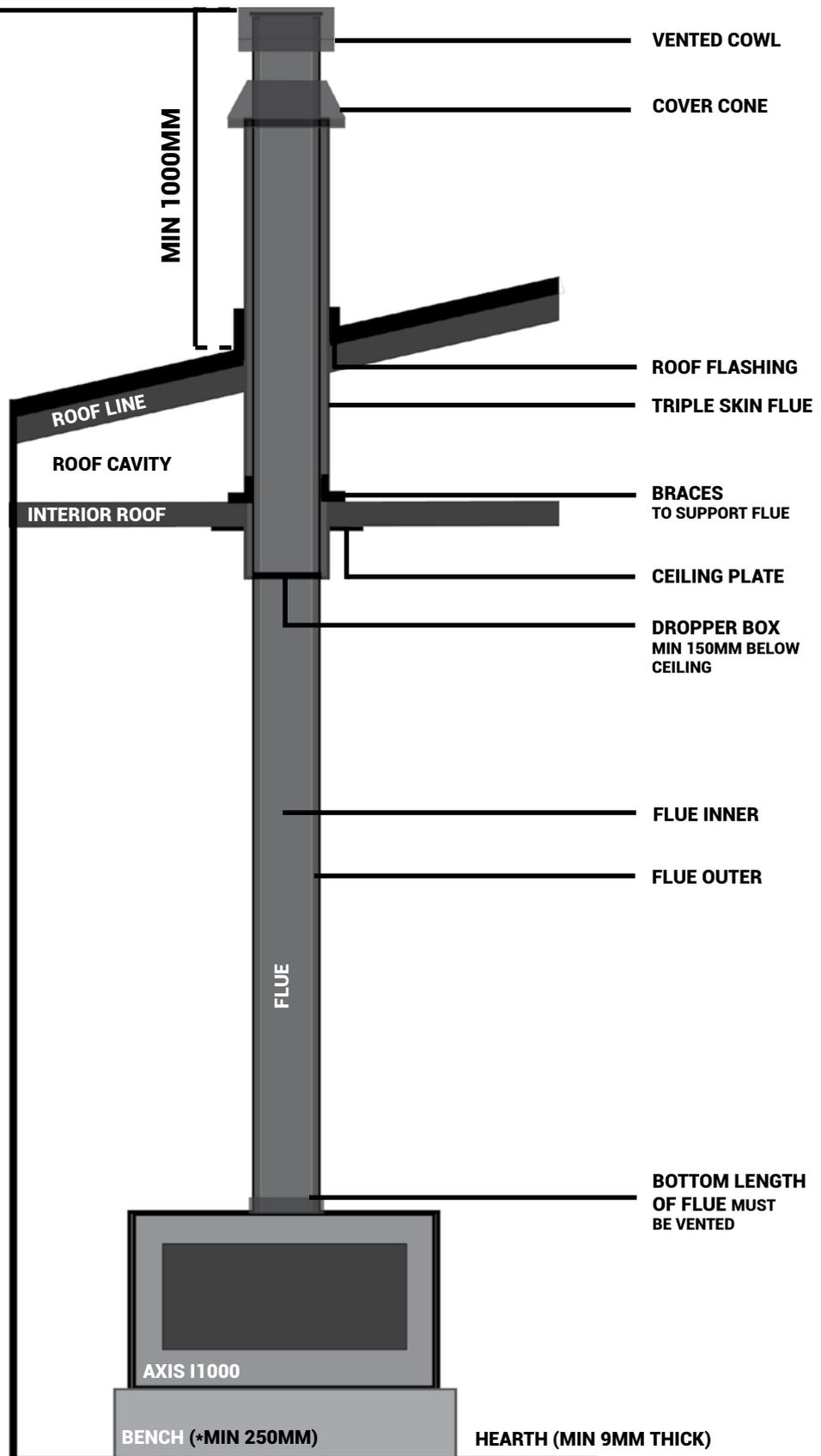
\*The appliance must be elevated a minimum of 250mm above the hearth (on a non combustible surface). If the heater is placed directly onto the hearth, the hearth dimensions required will be greater. Please refer to AS/NZS 2918:2001 as per the minimum for a non-tested appliance.
