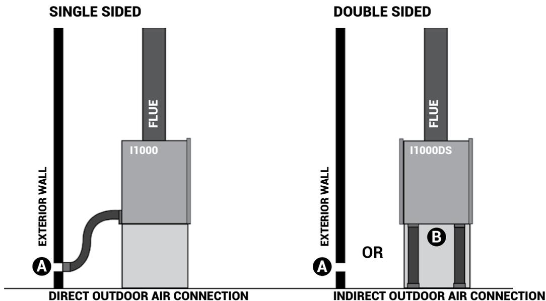
It is preferable to connect to outdoor air in order to optimise combustion control. Depending on specific building-related conditions (air tightness, presence of mechanically controlled ventilation, presence of a kitchen hood, etc).
