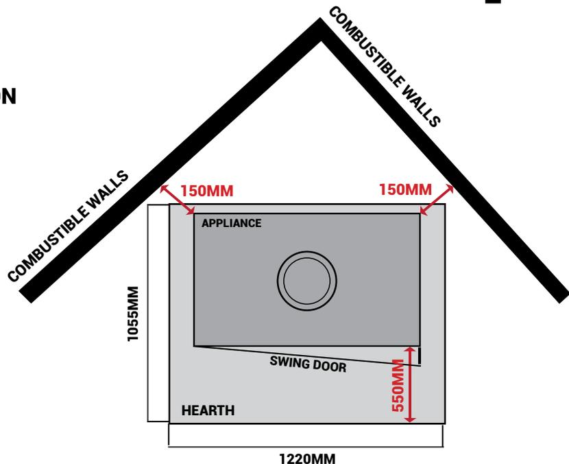
\*\*\*The appliance must be elevated a minimum of 250mm above the hearth(on a non combustible surface). If the heater is placed directly onto the hearth, the hearth dimensions required will be greater. Please refer to AS/NZS 2918:2001 as per the minimum for a non-tested appliance.
